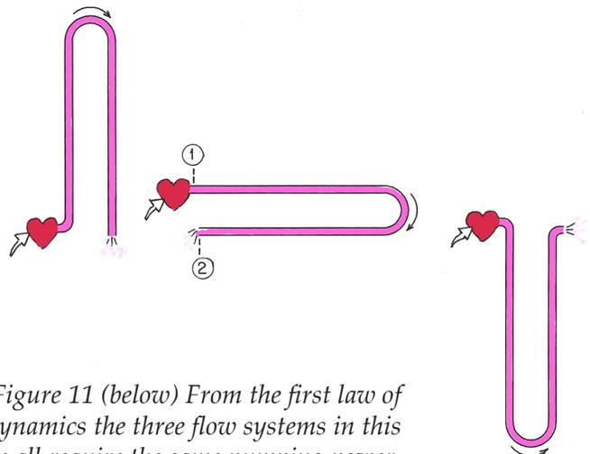
Figure 11 (below) From the first law of thermodynamics the three flow systems in this figure all require the same pumping power.
